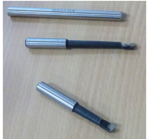
Boring head shown above left and various cutters right
